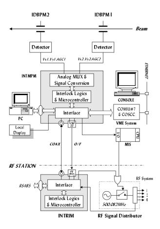
Figure 1: Schematics of the Interlock System
