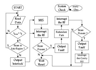
Figure 2: Flowchart of the main operation
