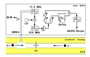
Figure 1: Schematic of BTM signal processing.
