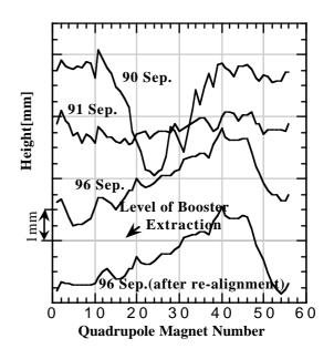
Figure 2. Height of the 56 quadrupole magnets from September 1990 through September 1996. Height is not absolute but relative value. Horizontal axis is the position of the quadrupole magnets. The first magnet is located in the injection section.
