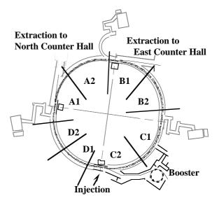
Figure 3. Foundations of the Main Ring Floor, complising eight separated plates.
