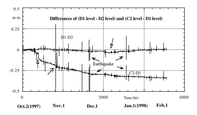
Figure 4. Time variation of the floor level differences of C2-D1, and that of D1 -D2. Floor level difference of C2-D1 changed rapidly (in fifty hours) by about 0.15 mm in the middle of October, 1997 and it increased gradually up to 0.35 mm for a few months. Many seismic vibrations were observed indicated by the dark arrows for example. At the end of October, as indicated by the simple arrow, the difference did not return to the one before earthquake.
