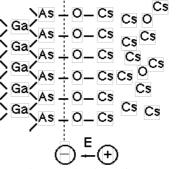
Fig. 2 : Microscopic view of NEA surface
