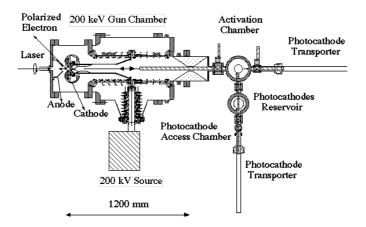
Fig. 4 : Schematic Plan View of 200keV Polarized Gun
