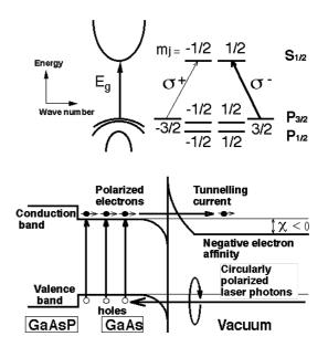
Fig. 1 : Principle of Strained GaAs-type PES
