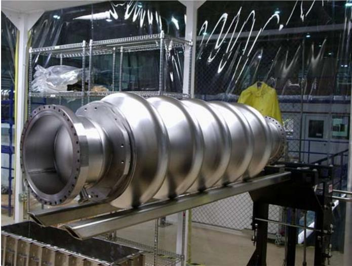
Fully damped “single mode” cavity at 703.75 MHz
