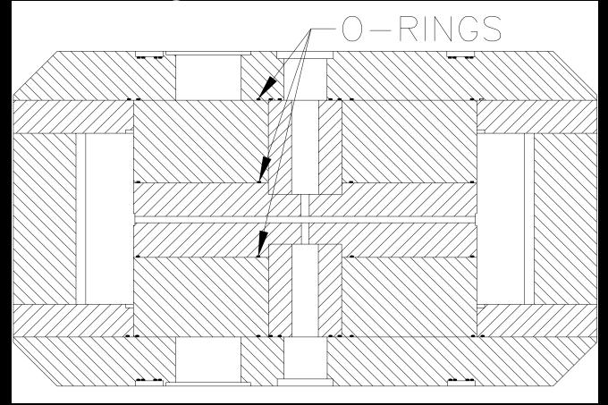
Cyclone 30 magnet steel & o-ring arrangement. O-ring replacement requires disassembly of the cyclotron magnet steel. This is particularly onerous for replacement of a lower-half o-ring. Special care must be taken to ensure that the relatively soft magnet steel does not bind. Fasteners and dowels are not shown.
