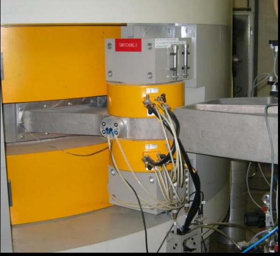
Cyclone30 switching magnet with shared return yoke with cyclotron. This design makes simultaneous dual extraction difficult.
