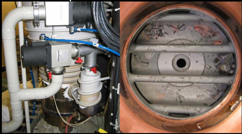
Cyclone30 ISIS is diffusion pumped. This introduces hydro-carbons into the ion source vacuum environment. Filament life-time decreases to ~80 hours, and H<sup>-</sup> production drops. Thick deposits (2mm to 3 mm) form on the source chamber walls. Debris drops onto the plasma electrode, and can fall through aperture to next lenses, buncher or inflector. 3/12/2007
