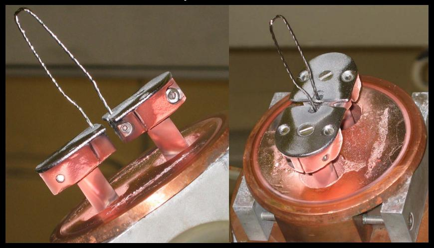
Hairpin tungsten filament and exposed support posts. The backplate has two cusp magnet rows
