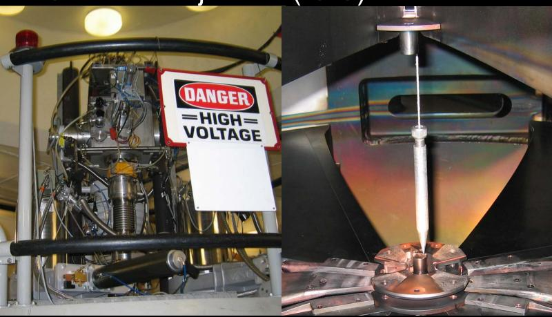
**ISIS** mounted on the moveable upper half of Cyclone30 with a cantilevered support. ISIS is moved each "lid-up" maintenance, and with a springy cantilevered support ISIS can become misaligned and requires correction as shown in RHS.
