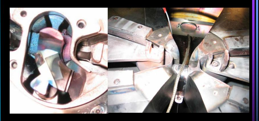
Cyclone30 inflector entrance with open ground enclosure, and no entrance collimator for beam diagnostic information. Right hand image shows dee bottoms in centre region, and hand connected high voltage cables for the inflector electrodes.
