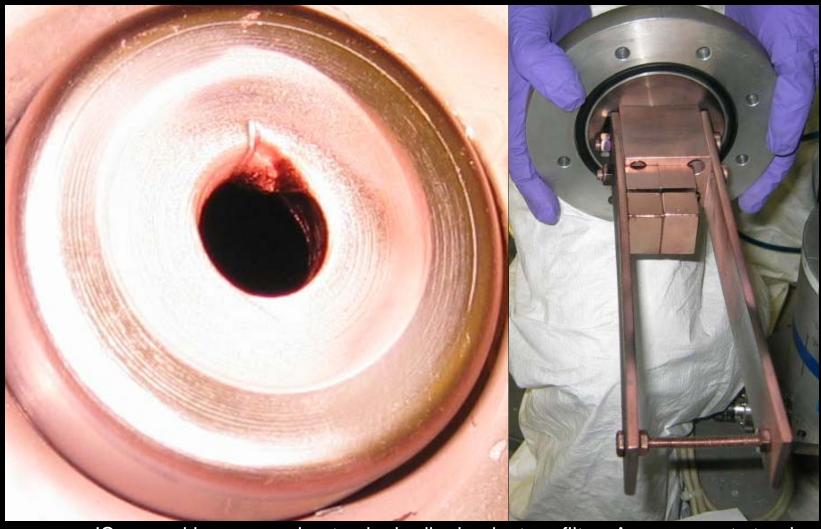
IS ground lens wear due to single dipole electron filter. A permanent steering magnet is used to correct beam steering introduced by the filter.
