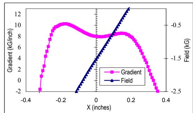
Figure 1: Field and gradient across a magnetic channel.
