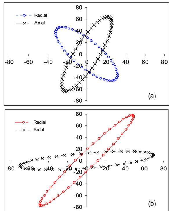
Figure 4: Phase space ellipse at (a) deflector entry (b)  $M_9$  Slit for ions with  $Q/A=0.5$ ,  $T/A=56$  MeV/n,  $B_0=31.08$  kG.
