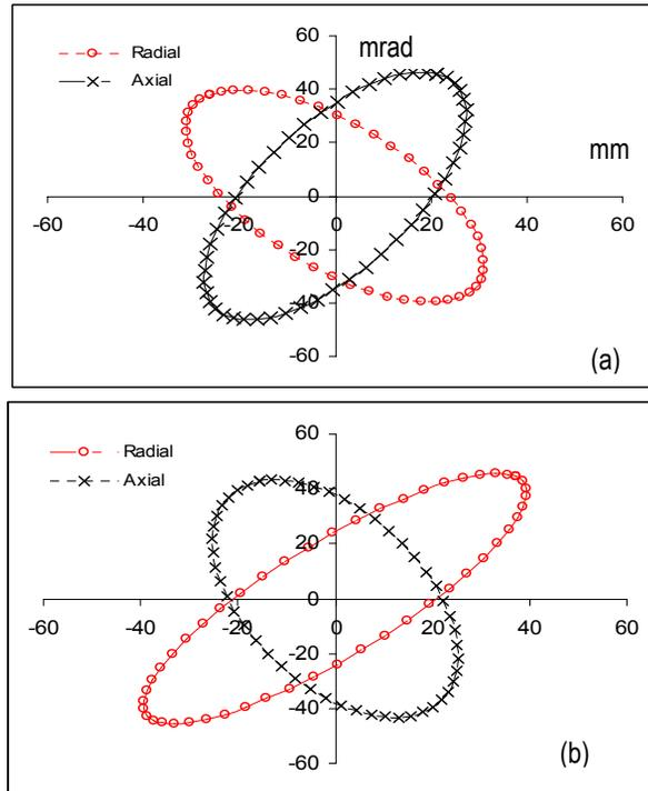
Figure 3: Phase space ellipse at (a) deflector entry (b)  $M_9$  Slit for ions with  $Q/A=0.25$ ,  $T/A=20$  MeV/n,  $B_0=38.3$  kG.
