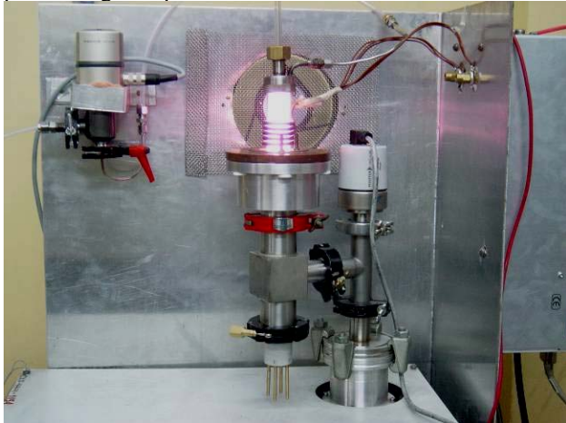
Figure 2: ICP ion source operating with 100W of RF power at 0.01 torr pressure.
