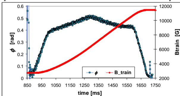
Figure 5: Cavity-to-beam phase  $\phi$  and magnetic field measured by the LLRF system as a function of cycle time.
