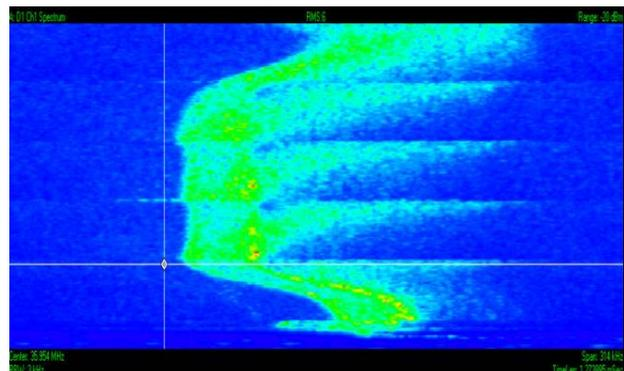
Figure 4: Spectrogram of the momentum cooling during stacking on the injection front porch. The vertical and horizontal axis denote time (1.6 s total from top to bottom); and momentum spread (1% full scale) respectively. There are 5 injections-cooling stacking sequences every 300ms
