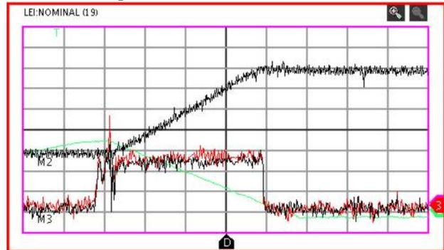
Figure 3: A typical multiturn injection in LEIR ( $50\mu\text{s}/\text{div}$ ). The green trace is the current of one of the 4 orbit bumpers, the red and black close traces are the injection current ( $10 \mu\text{A}/\text{div}$ ) and the black ramping trace is the accumulated current ( $270 \mu\text{A}/\text{div}$ ).
