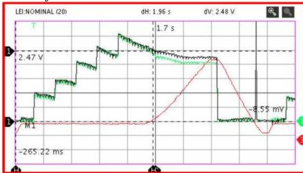
Figure 2 : The "nominal beam" in LEIR(400ms/div). The red trace is the main bending field, the green and black traces are the beam current with 5 injections ( $1.9 \cdot 10^8$  ions/div). Note the increased losses rate after each injection. About  $9 \cdot 10^8$  ions are present before acceleration and more than  $7 \cdot 10^8$  remain at extraction.
