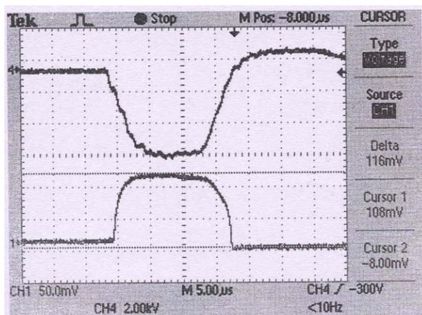
Figure 7: Voltage and current waveform of the electron gun measured using a divider and a FCT.
