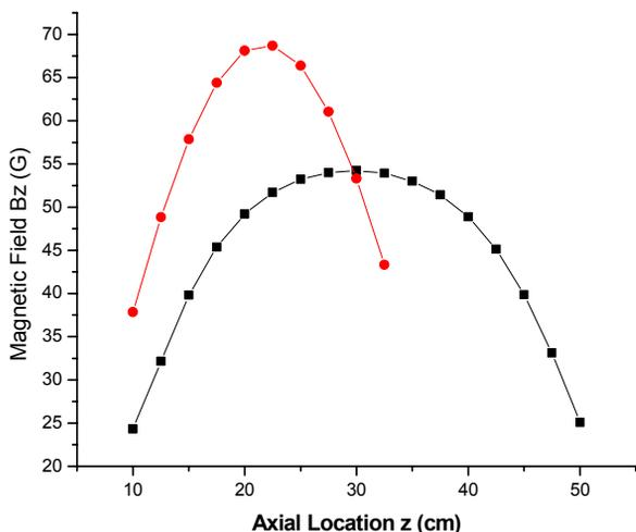
Figure 3: Axial field  $B_z$  versus  $z$  for S1 (•) and S2 (•).
