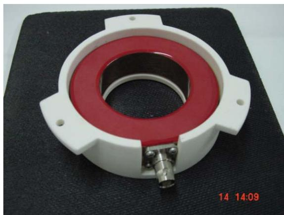
Figure 6: BCT and alumina enclosure
