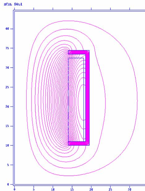
Figure 5: Field contour for solenoid S1.
