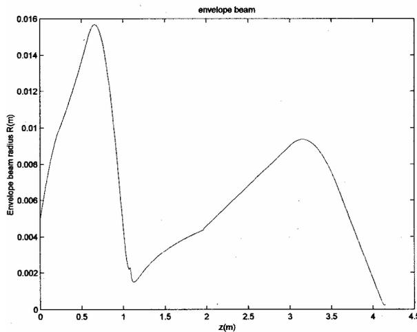
Figure 2: Beam envelope from EG to T: S1 ( $0 < z < 0.235$ ), D1 ( $0.235 < z < 0.585$ ), S2 ( $0.585 < z < 0.995$ ), D2 ( $0.995 < z < 1.087$ ), L ( $1.087 < z < 1.964$ ), D3 ( $1.964 < z < 3.014$ ), S3 ( $3.014 < z < 3.564$ ), D4 ( $3.564 < z < 4.15$ ).
