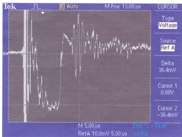
Figure 8: BCT signal for the beam current at the linac exit.
