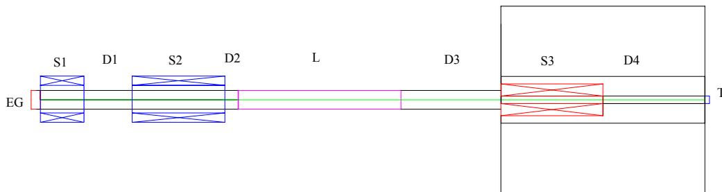
Figure 1: Schematic of beam transport elements: EG-Electron Gun, S-Solenoids, D-Drifts, L-Linac, T-Target.
