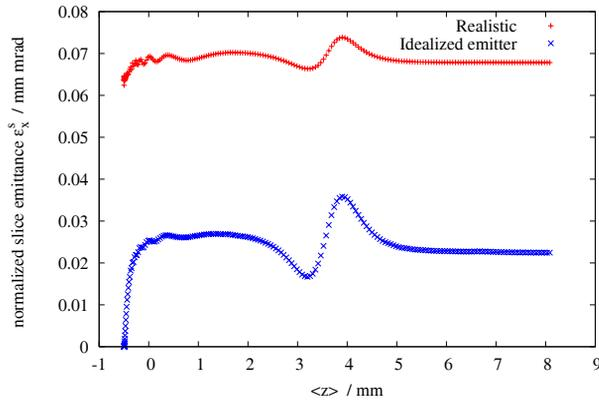
Figure 3: Evolution of slice emittance for homogeneous field emitter array ( $E_{acc} = 250 \text{ MV/m}$ ). Upper trace uses phases space computed from geometry in fig. 1, lower trace assumes ideal emitter with zero initial momentum spread.
