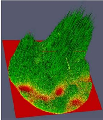
Figure 4: Stochastic transverse charge distribution at the exit of the gun ( $\beta = 1$ ,  $\zeta = 15 \mu\text{m}$ )
