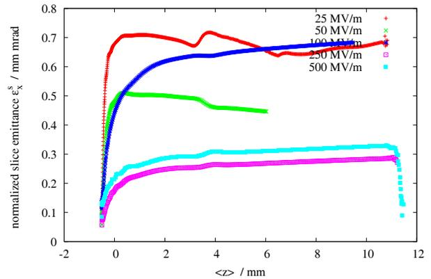
Figure 5: Evolution of slice emittance for an inhomogeneous field emitter array ( $\sigma = 2$ ,  $\zeta = 50 \mu\text{m}$ ) for various accelerating gradients. The initial current densities have different distributions (but same stochastic momenta) and are not perfectly comparable.
