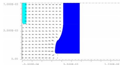
Figure 2: Gun geometry in cylindrical coordinates together with accelerating field.
