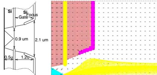
Figure 1: Geometry of double gated field emitter with beam trajectories ( $I_b = 0.5mA$ ).
