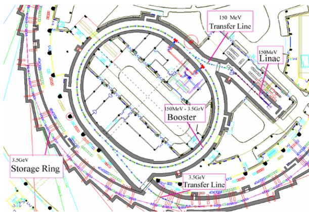
Figure 1: Schematic layout of SSRF injector
