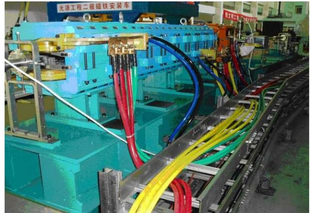
Figure 9: Test installation of a booster standard cell
