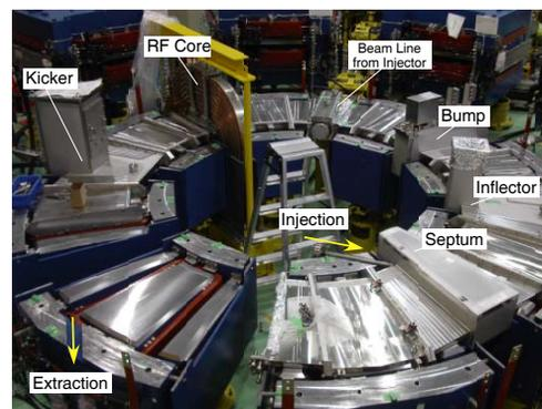
Figure 5: The booster FFAG under construction. DFD structure of the radial sector magnets can be seen in the front-left lattice. The remaining bump magnet and the septum for beam extraction are to be placed in the straight section before the lattice with beam extraction channel.
