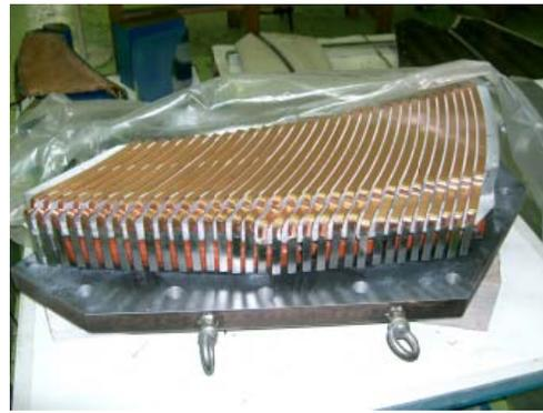
Figure 3: 32 trim coils attached to the pole piece of the injector.
