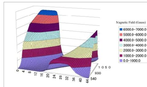
Figure 4: A typical FFAG magnetic field of the injector ring magnet with trim coils obtained by the field measurement.
