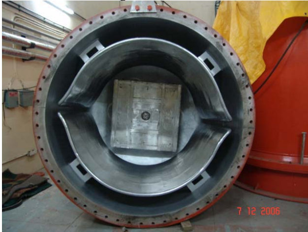
Figure 5: Rectangular Radiator Type Heat Exchanger inside the Top Portion of Accelerator Tank
