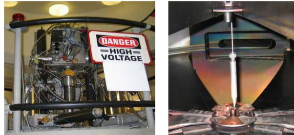
Figure 1: LHS shows ISIS on top of Cyclone30, and RHS shows ISIS out of alignment after several tank openings.
