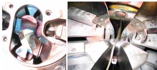
Figure 5: LHS shows inflector entrance with open ground enclosure. RHS shows dee bottoms in centre region.
