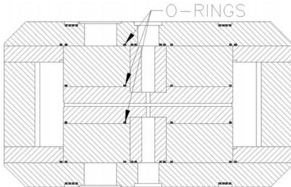
Figure 6: Cyclone30 magnet steel & o-ring arrangement. Fasteners/dowels are not shown. O-rings are not to scale.
