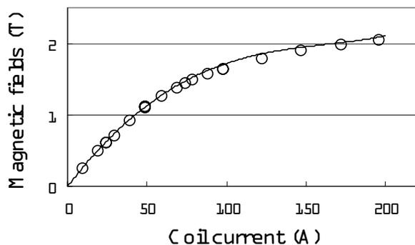
Figure 5: Magnetic fields  $B_z$  at the center of the air gap as a function of coil current(circle). Calculated magnetic fields are also shown(line).
