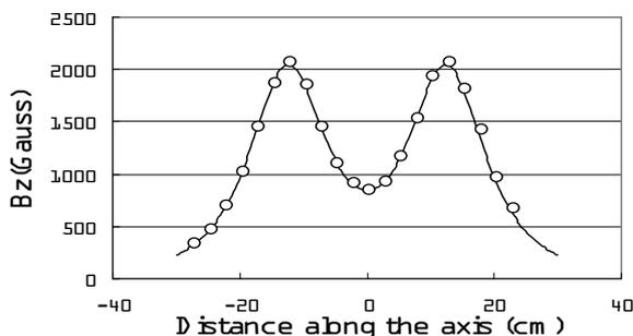
Figure 4: Longitudinal magnetic field  $B_z$  distribution along the central axis(points). The coil current is 100 A. Calculated magnetic fields are also shown(line).
