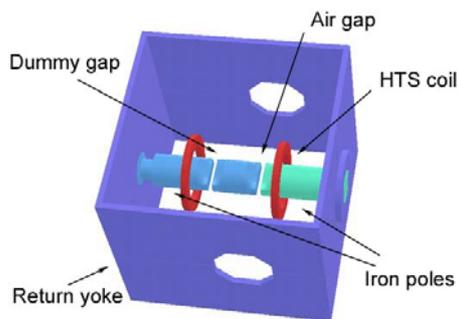
Figure 2: A 3D model of iron poles and return yokes. The positions of the HTS coils are also shown.
