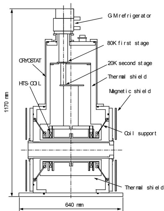
Figure 1: Cross sectional view of the HTS solenoid magnet.
