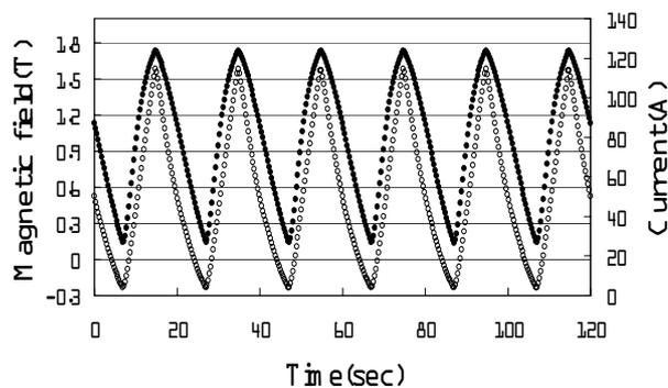
Figure 6: Observed magnetic fields on an AC operation(solid circle). The frequency is 0.05 Hz. Coil current measured at the current lead by a DCCT is also shown(open circle).
