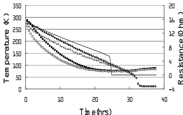
Figure 3: Temperatures and coil resistance as a function of a cooling time. Open and solid circles show temperatures of each coil. Temperatures of the second stage of the G-M refrigerator are shown in open triangles. Temperatures of a thermal shield(solid square) and the first stage of the refrigerator(open square) are also shown. Total resistance of two coils is shown by solid line.
