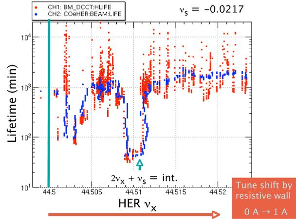
Figure 4: Synchro-betatron resonances in HER. The beam lifetime significantly shortened at the resonance  $2\nu_x + \nu_s = \text{integer}$ .
