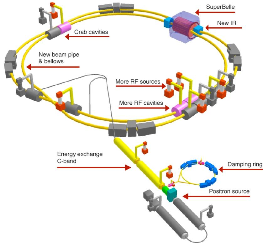
Figure 7: Schematic layout of SuperKEKB.
