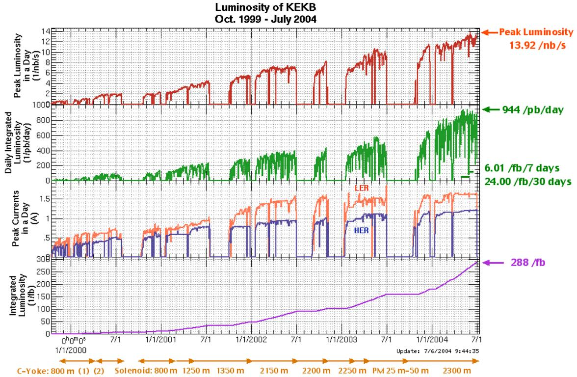
Figure 2: History of KEKB performance. 1) Peak luminosity in a day (1/nb/s) , 2) daily integrated luminosity (1/pb) , 3) peak currents in a day, and 4) total integrated luminosity. Arrows and numbers at bottom show the total length covered with magnetic field of solenoid and permanent magnets.
