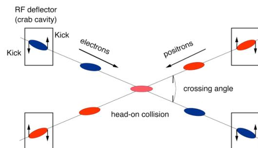
Figure 6: Schematic view of the crab-crossing scheme[5]. In the original design, we planned to install two crab cavities in each ring. Free spaces are reserved in the interaction region.
