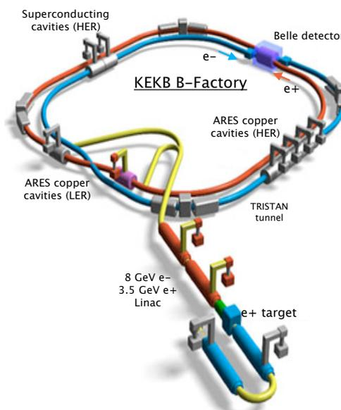
Figure 1: Schematic layout of KEKB.
