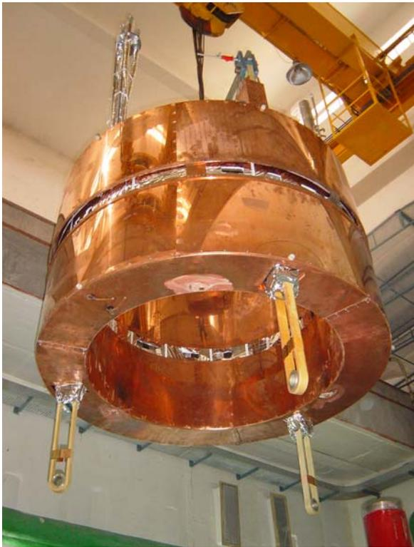
Figure 6: Cryostat bobbin with multilayer insulation and LN-2 cooled radiation shield. Support links are also shown.
