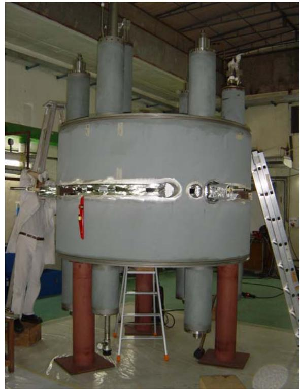
Figure 8: Final assembled cryostat without median plane inserts.
