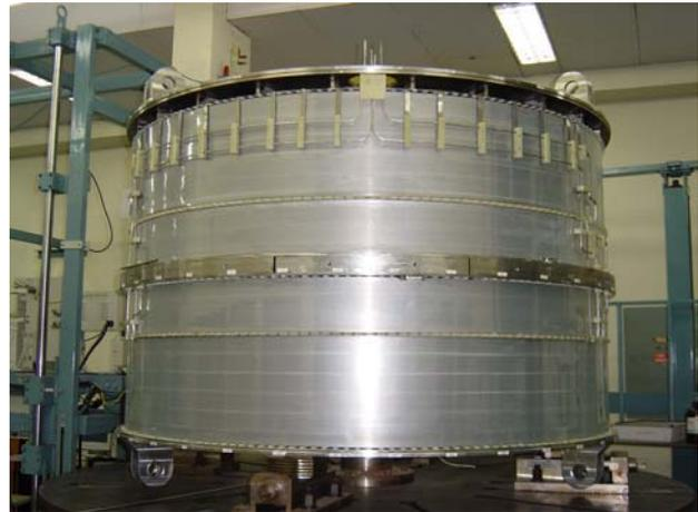
Figure 5: Superconducting coil for the cyclotron magnet
