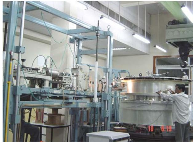
Figure 4: Superconducting coil winding in progress
