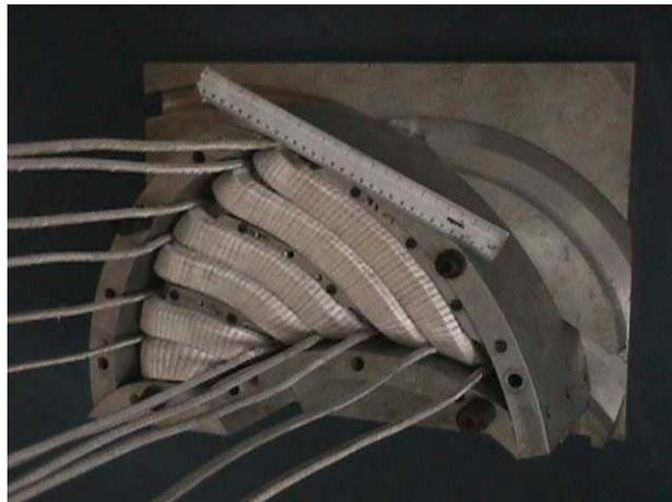
Figure 11: Trim coils wound on pole-tip.
