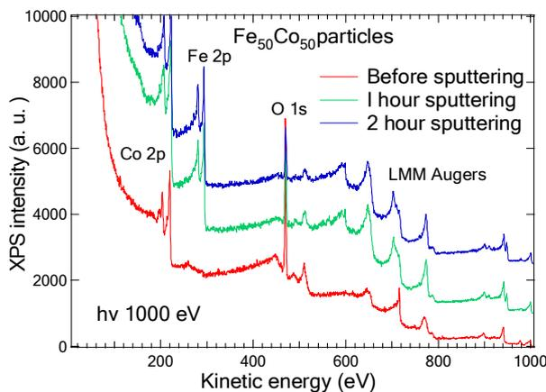
Fig. 10: XPS spectra of Fe/Co nanoparticles. Bottom curve was measured prior to sputtering, middle and top curve after 1 h and 2 h of sputtering, respectively.
