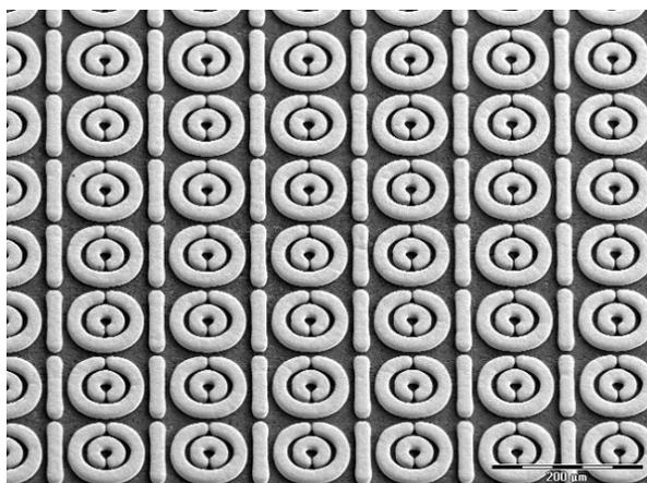
Fig. 7: Rod-split ring structures of Ni. Outer ring is 100 μm in diameter, spectral transmission is around 2.4 THz.
