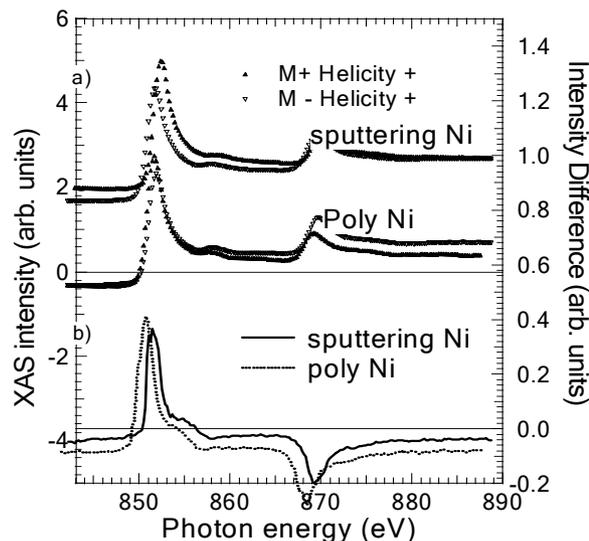
Fig. 11: XMCD spectra of sputtered Ni layers and standard polycrystalline Ni foils.
