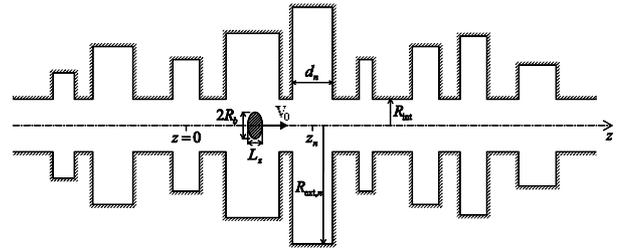
Figure 2: A finite-size bunch moving in vacuum at a constant velocity  $v_0$  along the axis of a structure with random size grooves.
