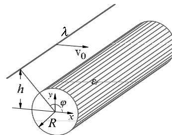
Figure 1: A line charge moving in the vicinity of a dielectric cylinder
