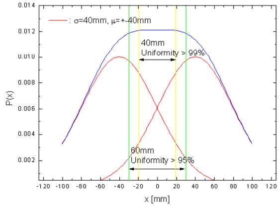
Figure 4: A dose density created by circular trajectory
