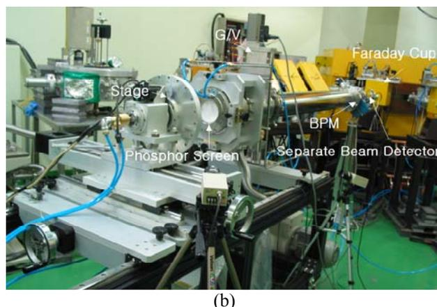
Figure 1: The 50MeV proton beamline
