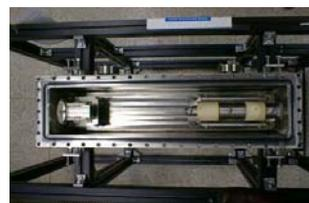
Figure 1: Bunching system of KIGAM.
