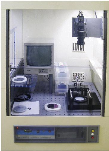
Figure 4: Inside view of the wafer bonding and IR inspection system.
