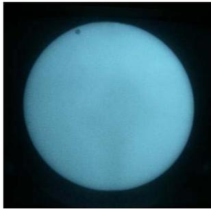
Figure 5: IR transmission image of directly bonded wafers with no void.
