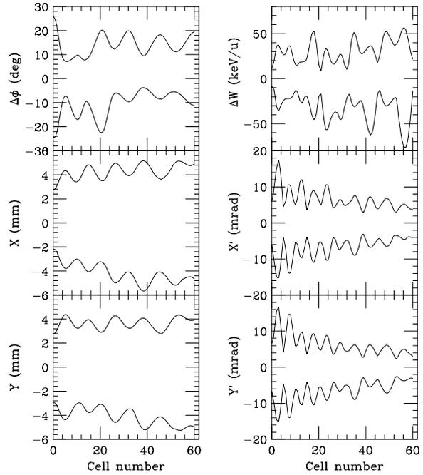
Figure 4: Beam envelopes for outmost particles as functions of the cell number.
