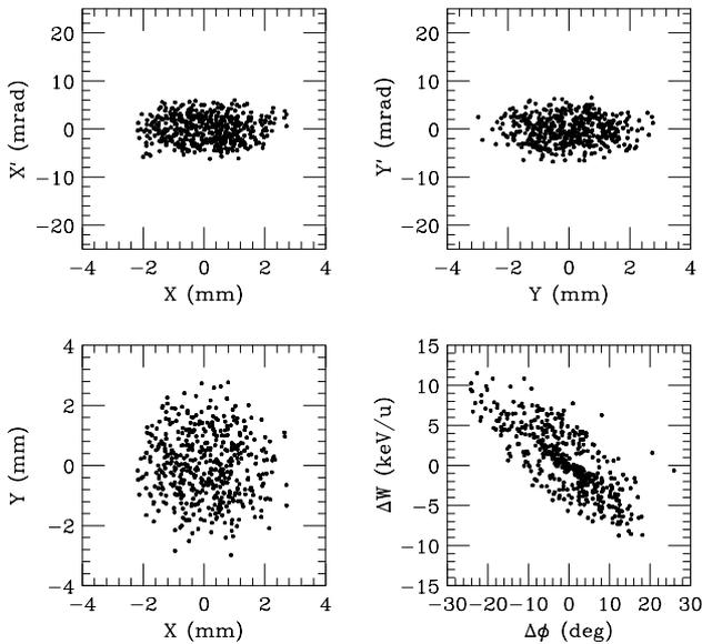
Figure 1: Phase space and X-Y distributions after the matching section. All the 482 particles extracted from the RFQ linac are plotted in the figures.
