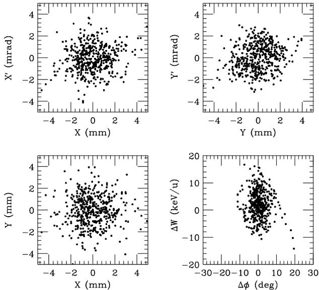
Figure 3: Phase space and X-Y distributions for the extracted beam from the APF linac. The 479 particles out of 482 were extracted. The corresponding transmission was 99%.
