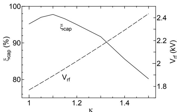
Figure 3: Capture efficiency and RF voltage as a function of dilution factor.
