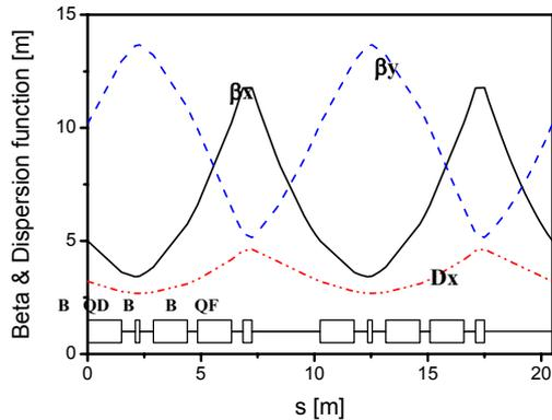
Figure 2: Beta function and dispersion function for two periods of the synchrotron lattice.
