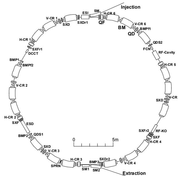
Figure 1: Layout of the synchrotron ring.
