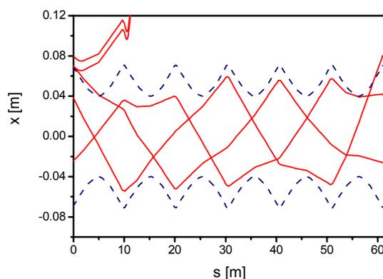
Figure 4: (a) Separatrix for each momentum of -0.05, 0.0, and 0.05 %. (b) Trajectory of last 3 turns and the extracted beam. Dashed curve represents envelope at injection including corrected COD.
