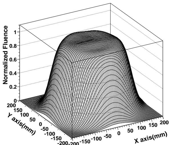
Figure 3: Typical results of the uniformity of the irradiation field. The field size is 220 mm in diameter and irradiation time is 1 s.
