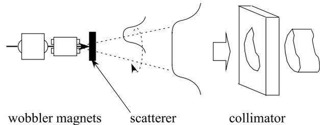
Figure 1: Schematic drawing of the wobbler-scatterer method. The wobbler magnets and the scatterer produce a uniform field and the collimator forms the field into a target shape for lateral direction.
