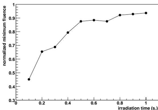
Figure 4: Uniformity of a 220 mm $\phi$  field as a function of the irradiation time produced by the spiral wobbler method. The fluence is normalized by the maximum fluence in the field.
