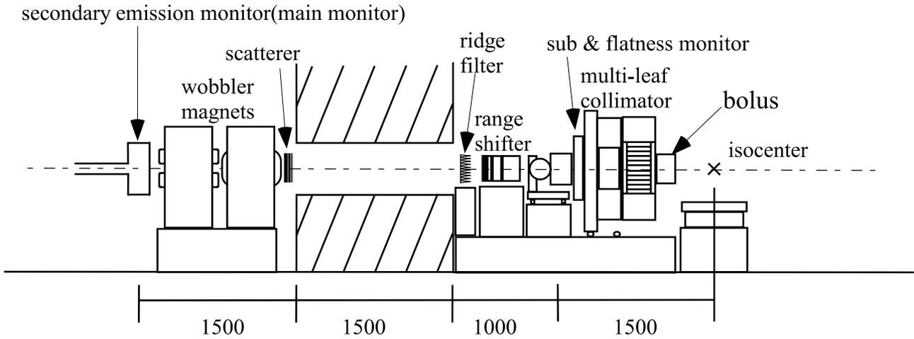
Figure 2: Schematic drawing of the compact irradiation port.
