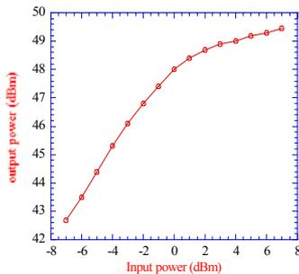
Figure 4: Experimental Drive Curve
