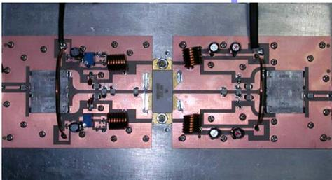
Figure 3: 4-stage 700MHz, 180W Solid State Big Power Amplifier
