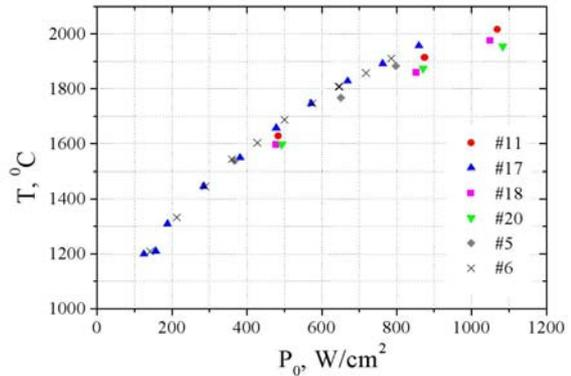
Figure 7: Maximum temperature of <sup>13</sup>C graphite vs the peak heating power density.
