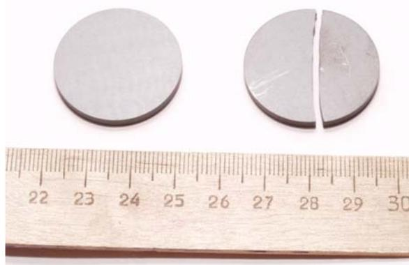
Figure 4: Picture of the boron carbide “Pure Tech” samples. Right – cracked sample after the test.
