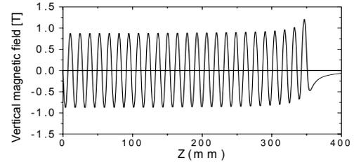
Figure 5: Vertical magnetic field as computed from eq. 1 for  $p=101$  and other parameters as given above.
