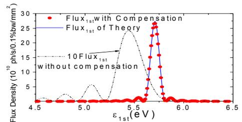
Figure 8: Fundamental radiation spectrum for the undulator with (circles) and without (dash-dotted) compensation coil in comparison to an ideal undulator (solid).
