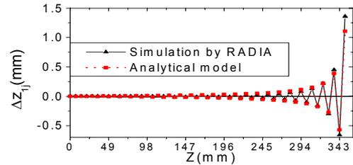
Figure 6:  $\Delta z_{1j}$  vs  $z$  from the analytical model and RADIA.
