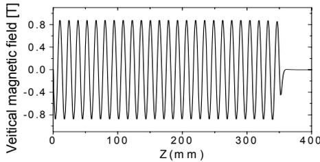
Figure 9: Vertical component of the magnetic field as computed from eq. 5 including the compensation field.
