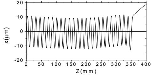
Figure 11: Beam trajectory along the undulator
