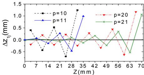
Figure 3:  $\Delta z_{1j}$  vs  $z$  for odd and even numbers of wire pairs. influence on the spectral output is depicted in Fig. 8 where the dash-dotted line displays the tenfold of the flux in the first harmonic of the  $p=101$  supramini while the solid line represents an ideal 50 period undulator. The curves were calculated using the SPECTRA7.0 code [6]
