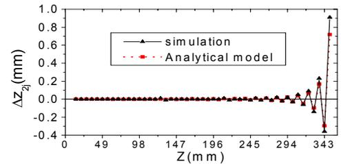
Figure 7:  $\Delta z_{2j}$  vs  $z$  from the analytical model and RADIA.
