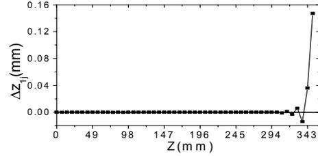
Figure 12: Mutual distance of adjacent field zeros  $\Delta z_{1j}$  for the compensated field of the  $p=101$  supramini.
