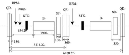
Figure 2: Schematic diagram for one cell
