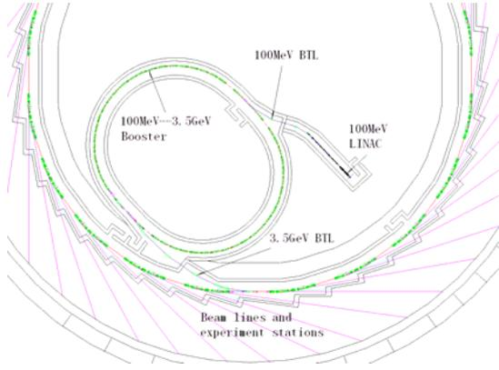
Figure 1: The Schematic layout of SSRF injector
