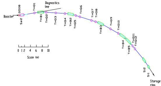
Figure 7: The Schematic Layout of BTS
