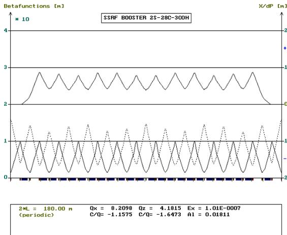
Figure 3:  $\beta$ -Function and Dispersion of Booster
