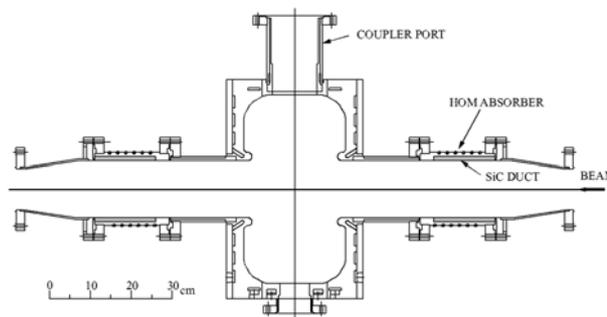
Figure 3: Cross section of the damped accelerating cavity for the PF storage ring.
