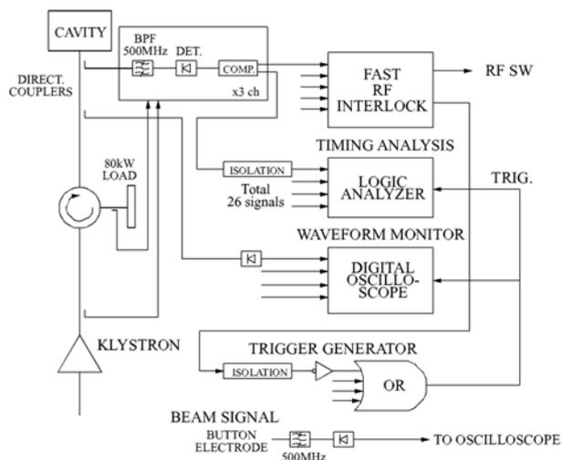
Figure 4: RF protection and its diagnostic system.
