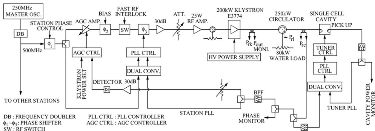
Figure 1: Block diagram of one of the four rf stations for the PF storage ring.
