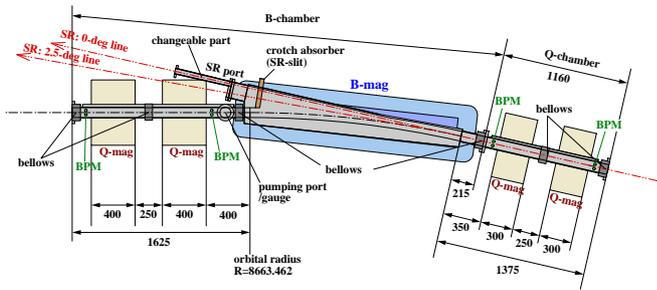
Figure 4: Conceptual chamber design.
