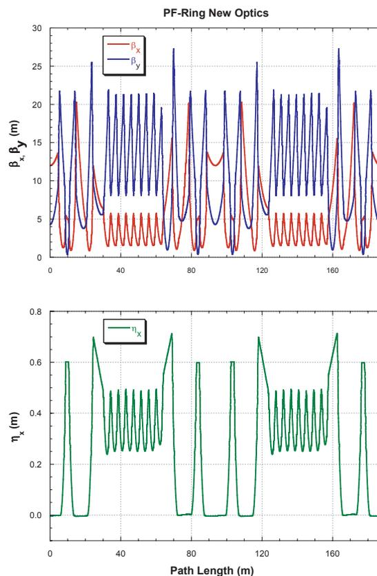
Figure 3: Optics for the straight-sections upgrade.
