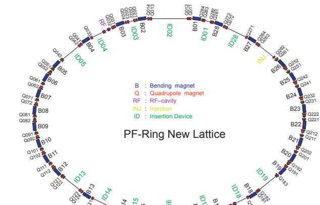
Figure 2: New lattice for the straight section upgrade project.
