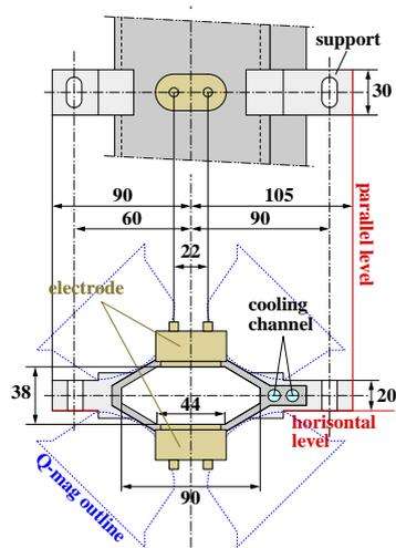
Figure 5: Design of beam position monitor.
