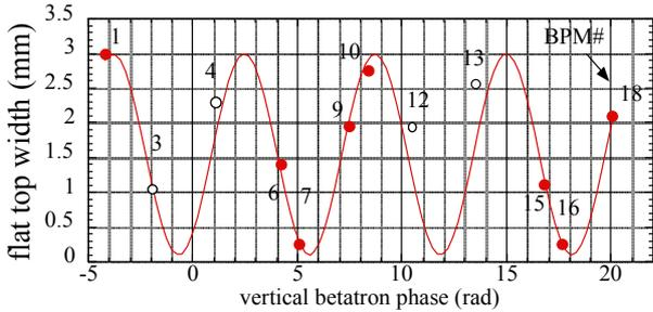
Figure 4: Flattop width of the aperture survey vs. the vertical betatron phase. The line is a 4th harmonic sinusoidal wave. The shaded circles and clear circles are critical locations face to SSS and LSS, respectively.
