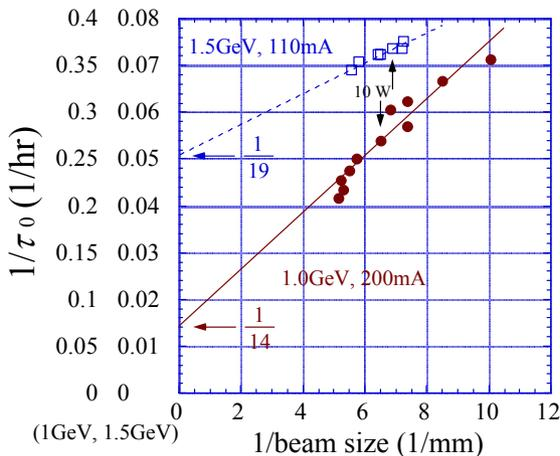
Figure 5: Vertical beam size ( $\sigma$ ) versus the beam lifetime at 1.0 GeV (circle) and 1.5 GeV (square). The points at  $[1/\text{beam size}] = 0$  are considered to be  $1/\tau_R$ .
