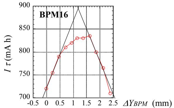
Figure 3: A typical result of the vertical aperture survey at 1.0 GeV. Vertical axis is the beam current times the lifetime. About 15% improvement of the lifetime was obtained by the 1.2mm displacement of vertical position at BPM nearby ( $\Delta Y_{BPM}$ ). The slope at the flattop was thought to be an effect of the spill of the local bump orbit.
