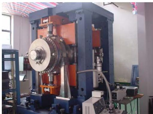
Figure 8: In-vacuum wiggler (4W2).
