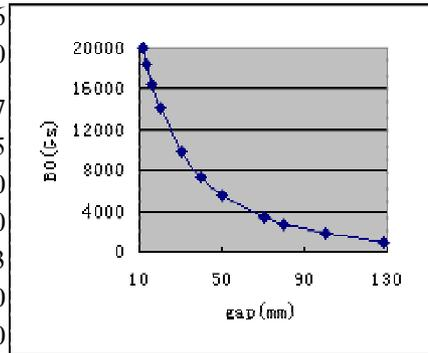
Figure 5: The curve of the magnetic field vs. gap.
