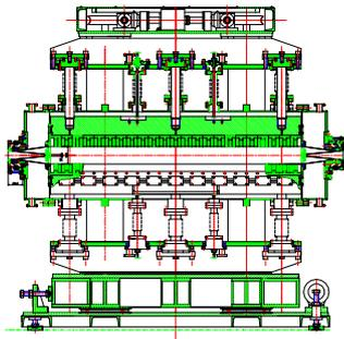
Figure 3: The mechanical diagram of the wiggler.
