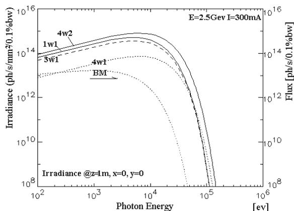
Figure 7: Irradiance calculated from wigglers at BEPC.
