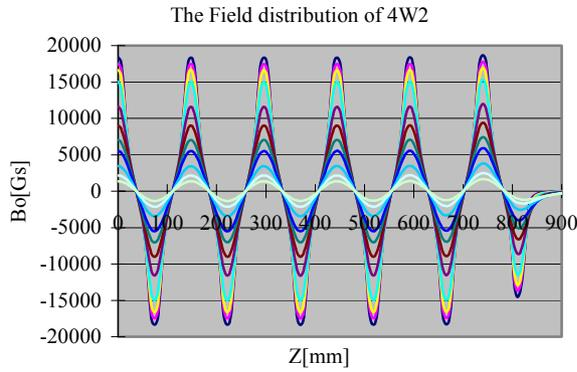
Figure 2: The magnetic field distribution at the mid-plane of 4W2 (only for half array).
