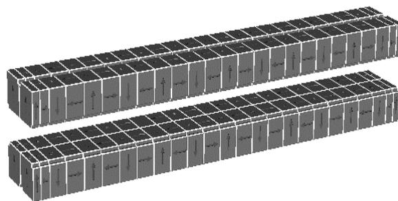
Figure 1: Four magnet arrays of the undulator.
