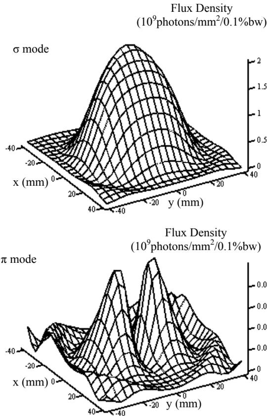
Figure 4: Flux density of the horizontal linear polarized radiation with the wave length 501  $\mu\text{m}$ .
