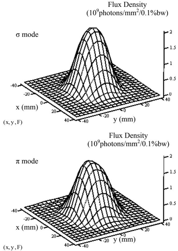
Figure 5: Flux density of the circular polarized radiation with the wave length 269  $\mu\text{m}$ .
