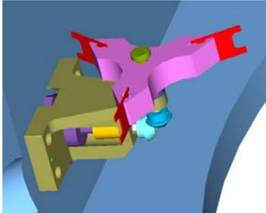
Figure 6 Carbon stripper foil holder
