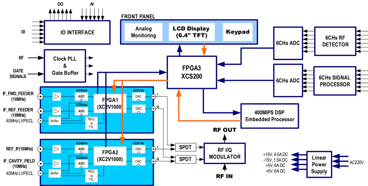
Figure 1: Simplified block diagram of the digital RF feedback system for PEFP 100MeV Proton LINAC
