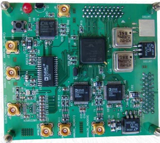
Figure 2: Photograph of AD/DA CORE BOARD
