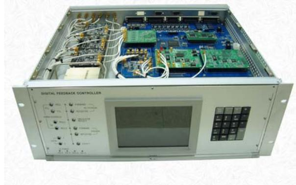
Figure 3: Photograph of the digital RF feedback controller for PEFP 100MeV Proton LINAC
