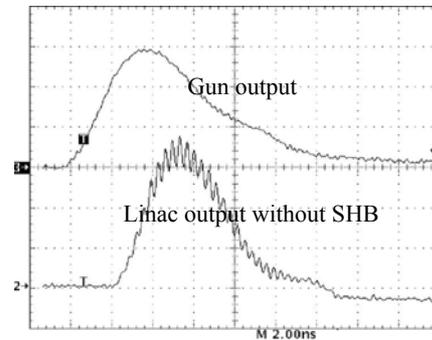
Figure 4: Long electron pulse at the exit of gun and the end of linac without SHB
