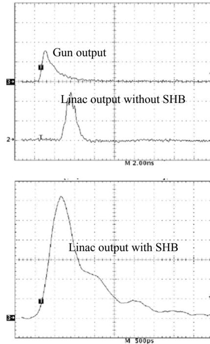
Figure 3: Short single electron pulse at the exit of gun and the end of linac with or without SHB
