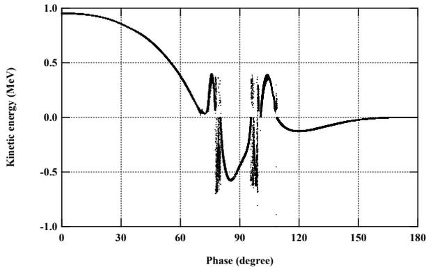
Figure 1: Kinetic energy gain plotted as a function of the initial RF phase of the electron.
