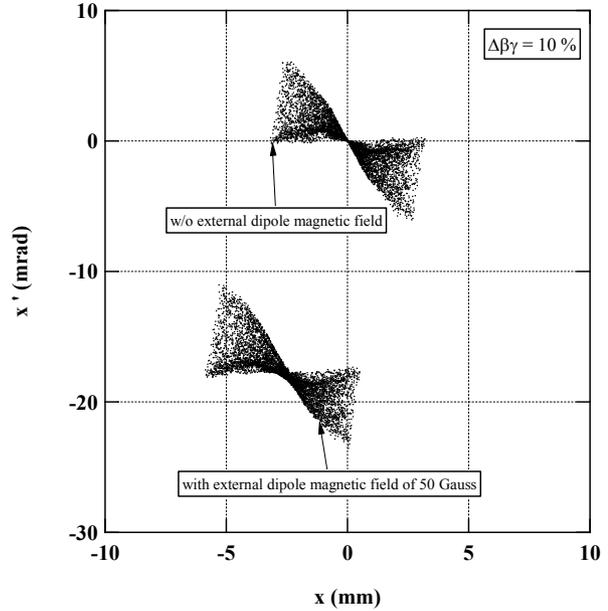
Figure 2: Transverse phase-space distribution at the RF gun exit.
