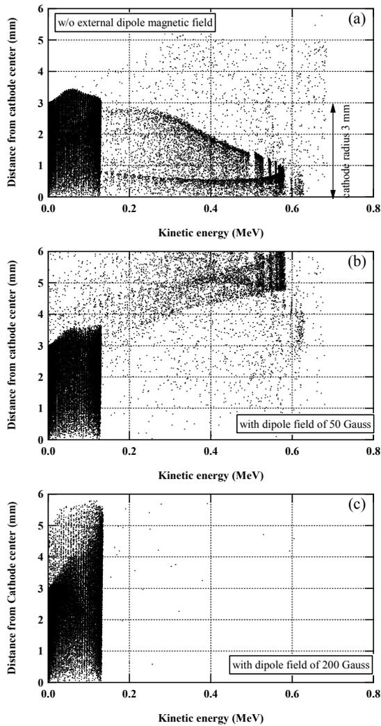
Figure 3: Radial distribution of the back-streaming electrons on the cathode plotted as a function of the kinetic energy.
