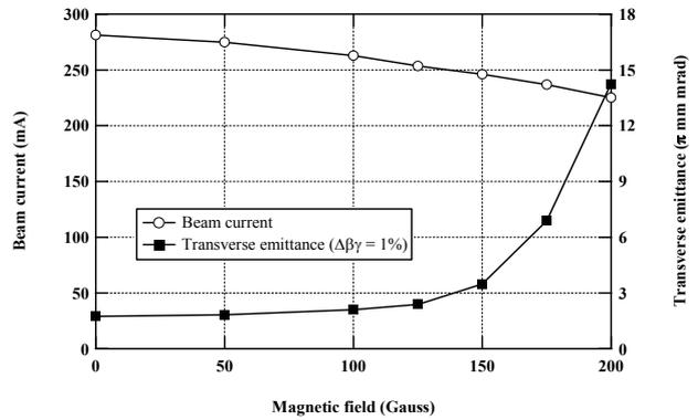
Figure 4: Variations of the transmitted beam current and the transverse emittance by changing the strength of the dipole field.
