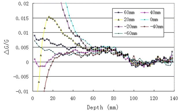
Figure 6: Different field along the depth orientation in the symmetry plane. (Different set of data shows the different horizontal position measured.)
