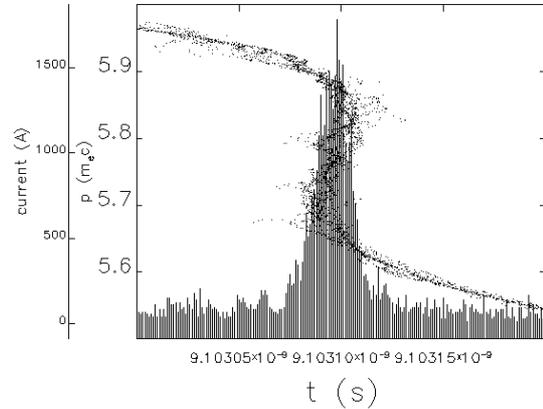
Figure 5: The particle distribution in longitudinal space at GTL exit (by ELEGANT [7])
