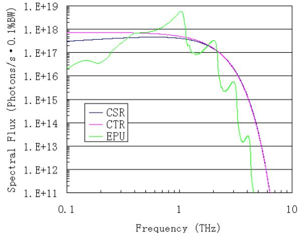
Figure 8: The THz radiation brightness from CTR, SR and EPU.
