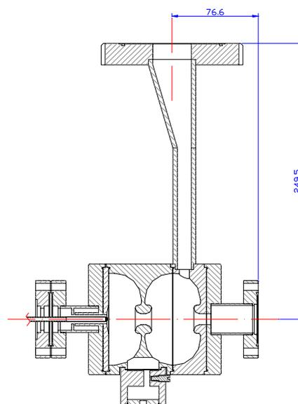
Figure 1: Cross section of the RF gun
