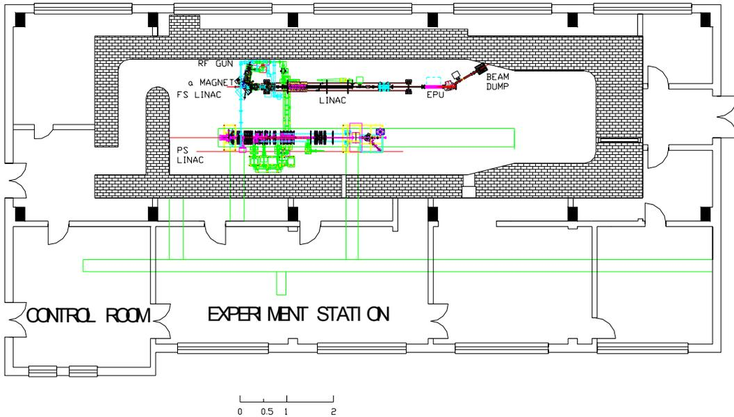
Figure 9: Layout of the THz source facility.
