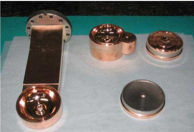
Figure 2: Some parts of the RF gun. (The coupler and the side cavity has been brazed to the first cavity and the second cavity respectively)
