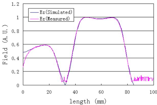
Figure 3: The field profile of RF gun at  $\pi/2$  mode.
