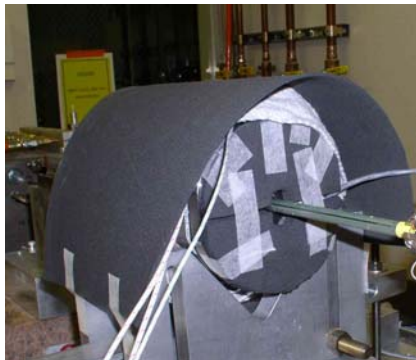
Figure 5: PMQ, covered with foam sheet, measured with rotating coil[3].
