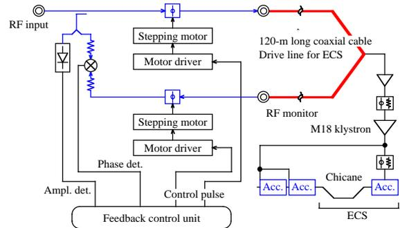
Figure 5: Diagram of PLL system for long drive line.
