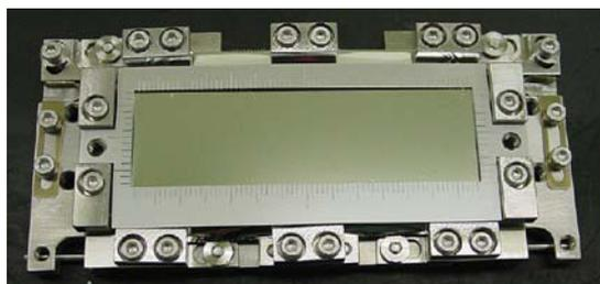
Figure 7: OTR screen to monitor beam energy.
