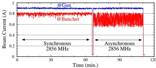
Figure 4: Stability of single-bunched beam.
