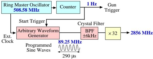
Figure 3: Block diagram of RF reference generator.
