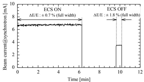
Figure 6: Stability of high-current 40 ns beam injection.
