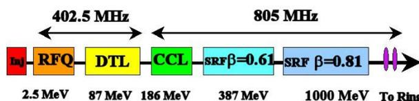
Figure 2: Schematic layout of the linac structure.
