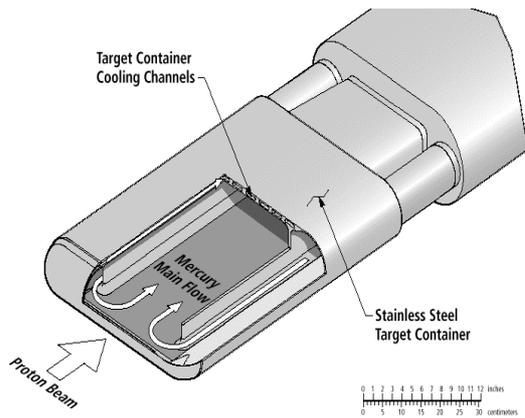
Figure 11: The SNS neutron producing Hg target
