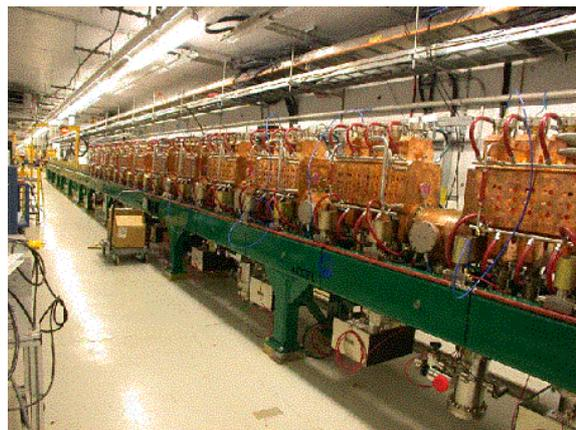
Figure 5: CCL RF module 1 in the SNS tunnel.
