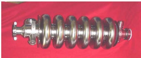
Figure 6: SNS 6-cell medium beta cavity.
