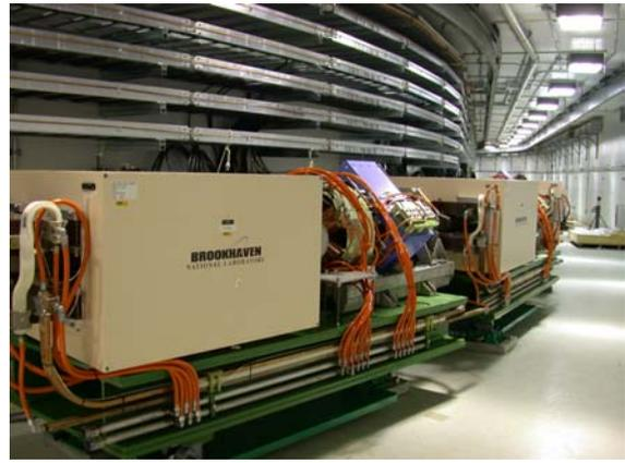
Figure 10: Ring half cell installed in the SNS tunnel.
