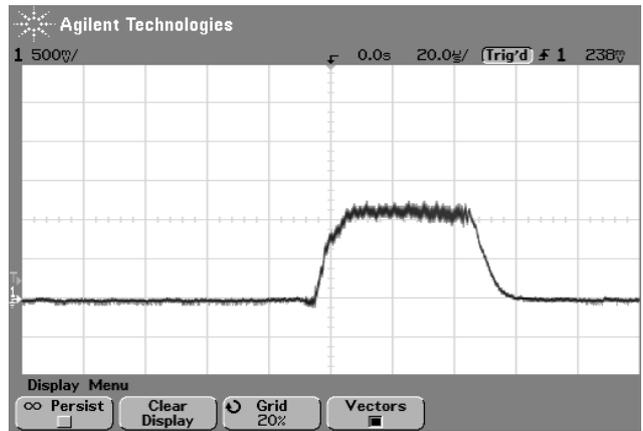
Figure 4: Pulsed beam signal from Faraday cup (10 $\mu$ s/div., 1 $\mu$ A/div.)
