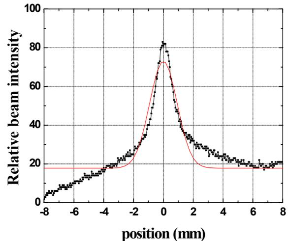
Figure 1: Intensity profile obtained along the vertical line around the proton beam.
