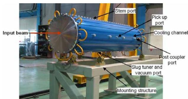
Figure 5: The fabricated DTL tank (1 section)
