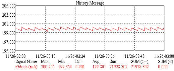
Figure 2: Zooming the top-up injection. The injection interval is 2 minutes, maximum beam current is 200 mA and the current bin is  $\sim 0.6$  A.
