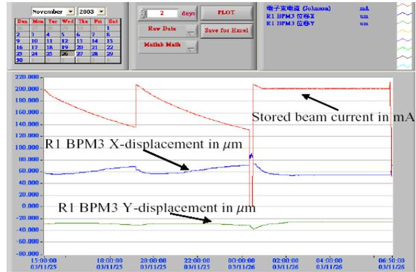
Figure 4: Recorded absolute position displacement in vertical and horizontal directions of BPM during decay and top-up mode.
