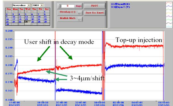
Figure 5: Reading of BPMs in the storage ring indicates the current-dependent effects. The reading of beam position can drift as much as 3-4  $\mu\text{m}$  in one user's shift, if the effect was calibrated correctly.
