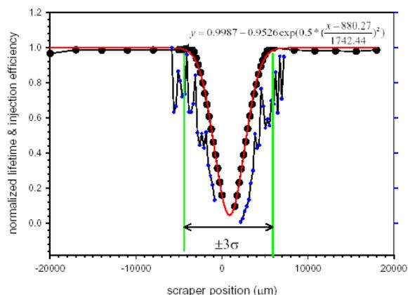
Figure 7: Vertical scrapers were used to measure the minimum aperture size of the ring without affecting the beam lifetime and the effect on injection efficiency.
