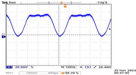
Figure 3: Filling pattern at the beginning of top-up injection. Filling pattern is identical to the shown pattern at the end of the test.
