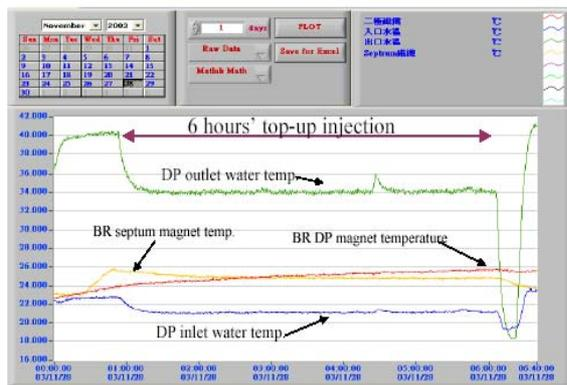
Figure 6: The temperature readings of dipole magnet and septum core under intermittence operation mode of injector at TLS.
