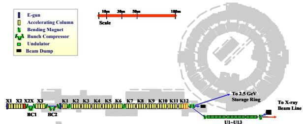
Figure 4: PAL-XFEL compression and acceleration.
