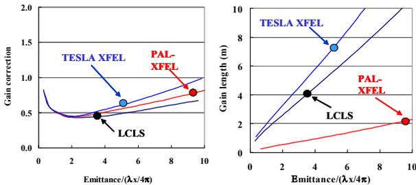
Figure 2: Gain length and gain correction factor.
