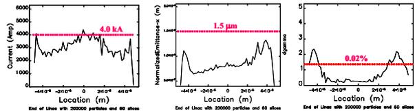
Figure 6: Beam quality at the end of linac.
