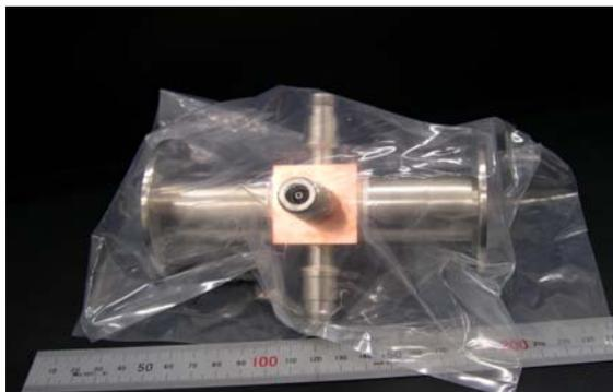
Figure 3 The prototype assembly of 4-Buttons type PU of the BPPM.
