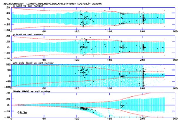
Figure 3: Configuration plot of the beam obtained by PARMTEQM with 10,000 particles.
