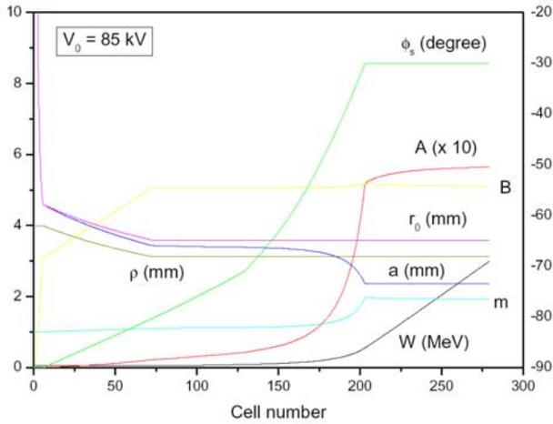
Figure 1: PEFP 3MeV RFQ Design Parameters: synchronous phase ( $\phi_s$ ), accelerating efficiency (A), focusing efficiency (B), mid-cell aperture radius ( $r_0$ ), minimum radius curvature (a), transverse curvature radius of the vane-tip ( $\rho$ ), modulation (m), and particle energy (W).
