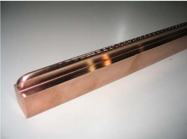
Figure 5: Vane end for machining check.
