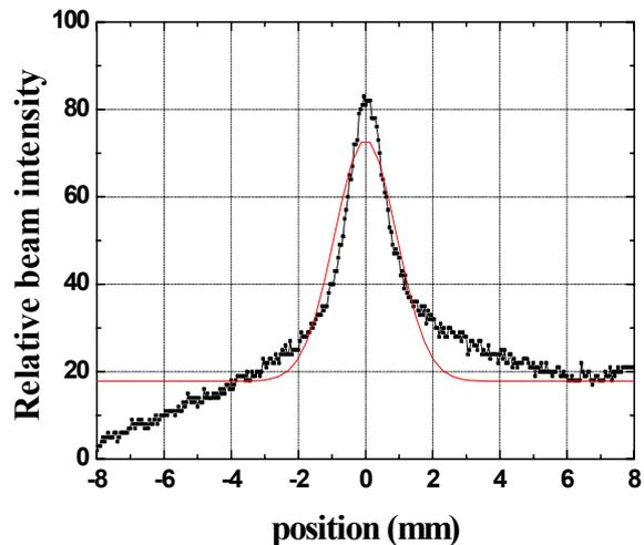
Figure 4: Intensity profile obtained along the vertical line around the proton beam.
