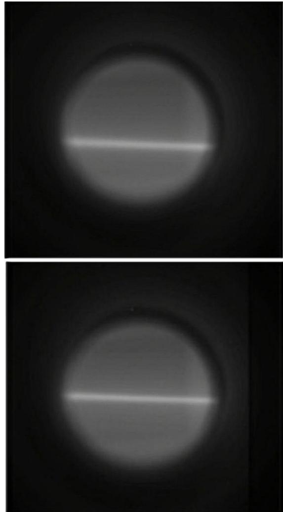
Figure 3: Two beam images, measured with the CCD beam profile monitor: (a) before operating the steering magnet and (b) after steering correction.
