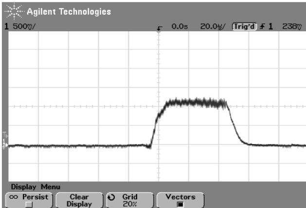
Figure 4: Pulsed beam signal from Faraday cup (10µs/div., 1µA/div.)
